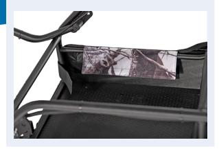
6 Secure the cover with a screw behind the chain protection.
