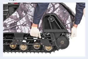
4 Secure the cover and the front mud flap with screws.
