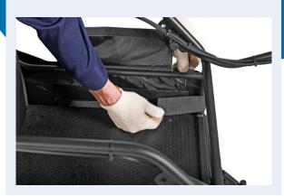
8 Install the cover support bracket under the cover and secure it with screws on the left, right and upper sides.
