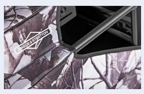
9 Secure the cover with screws near the chain protection.
