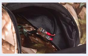
10 Connect the lighter outlet. The red wire with white stripe must be connected to the positive connector of the lighter outlet.
