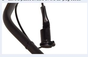
3 Cut and remove the heat-shrinkable isolator sleeve from the lighter outlet.
