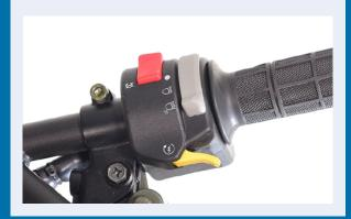
1 Turn the switch on the steering bar switch in "off" position.
