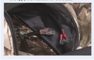
9 Connect the lighter outlet cleat with the heater cleats.
