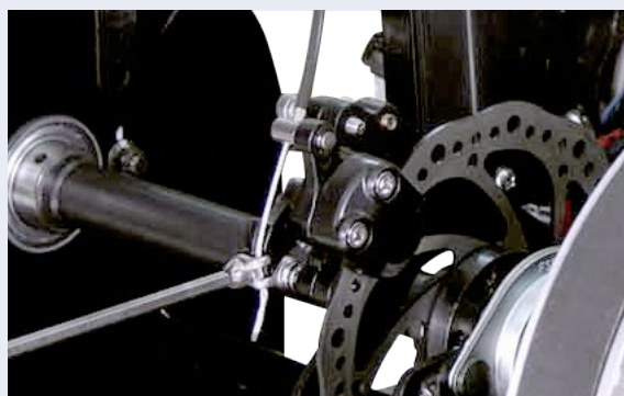
11 Loosen the screw, which fixes the brake cable to the brake caliper and disconnect the brake cable.
