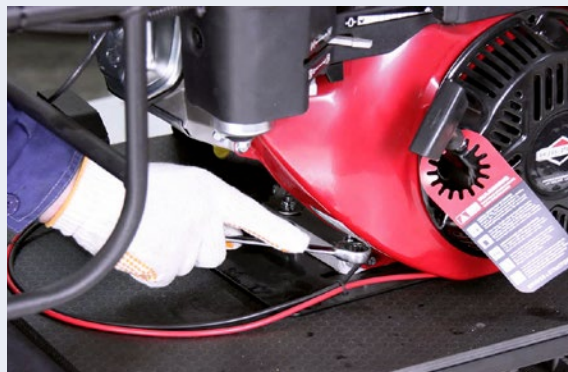
9 Unscrew 4 engine-securing M8 nuts and take off 2 guide bushings.
